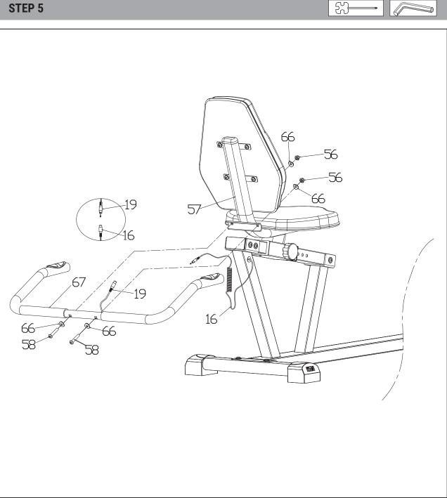
Securely attach the rear handlebar (67) to the saddle support set (57) using the screw (58), curved washer (66), and cap nut (56), and tighten them with a wrench.
