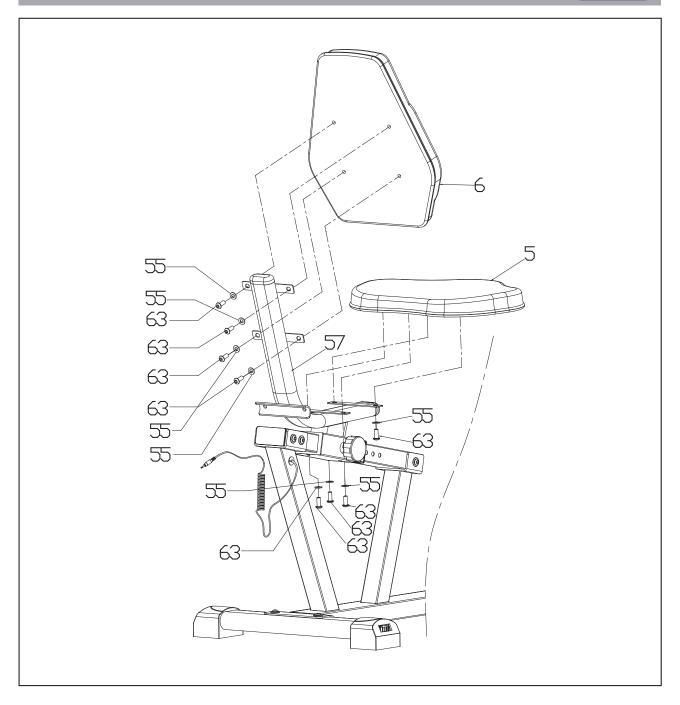
Attach the saddle (5) and back cushion (6) to the saddle support set (57) using screws (63) and flat washers (55), as indicated separately, and securely tighten them with a wrench.
