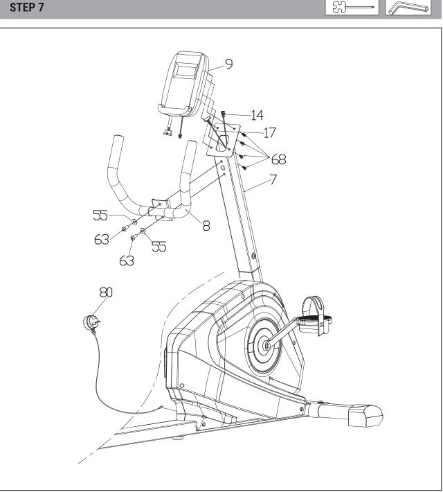
Attach the handlebar (8) to the front post (7) securely using a flat washer (55) and screw (63), ensuring a tight fit.
