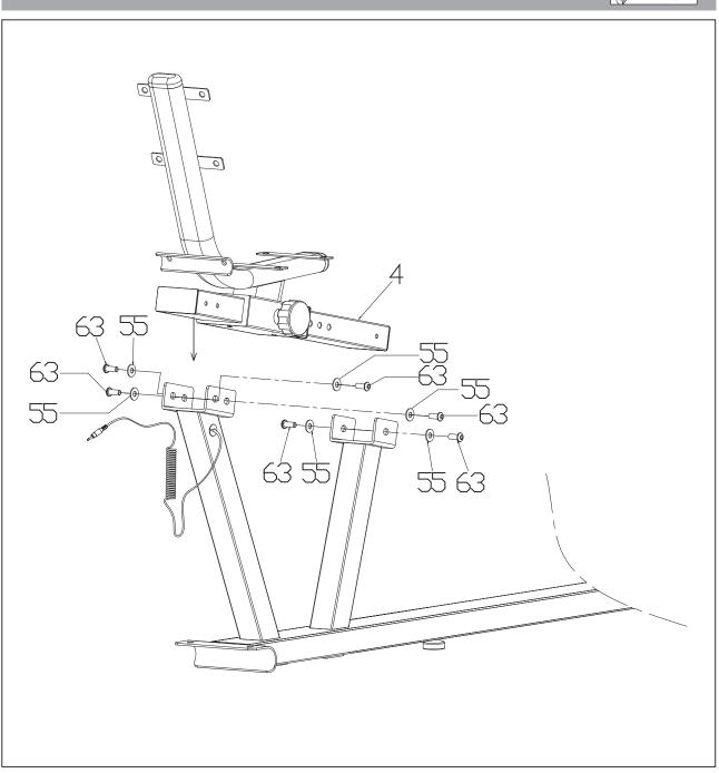
Loosen all the screws (63) and flat washers (55) on the saddle adjusting tube (4) using the wrench, and ensure they are safely stored.
