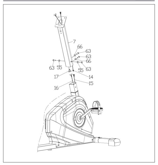
Carefully connect the console wires (14&15) together. Ensure the sensor wires (16&17) are connected correctly. Straighten all pins before connecting wires 14 & 15 and 16 & 17 to prevent console malfunction.
