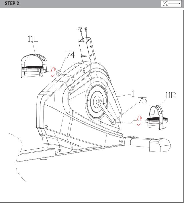
Securely attach the left pedal (11L), indicated with "L," to the left side of the crank (74), also marked with "L," using a spanner in an anticlockwise direction.
