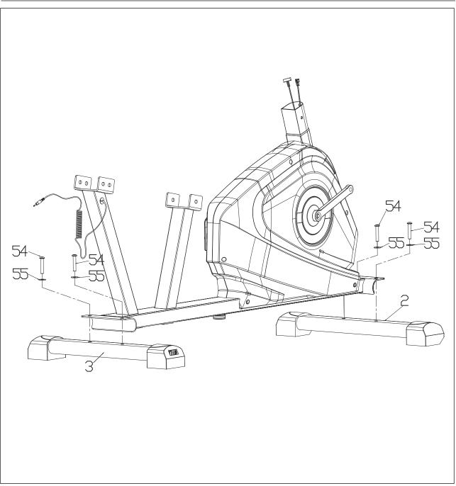
Remove all the screws (54) and flat washers (55) from the front stabiliser (2) and the rear stabiliser (3) using the Allen key, and store them securely.
